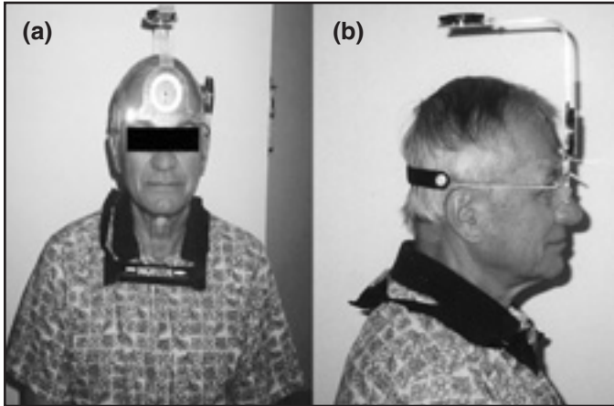
Figure 1. Frontal (a) and lateral (b) view of a subject wearing the CROM instrument.
